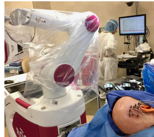
Stereo-Electroencephalography. The highly precise ROSA robot is used to guide the implantation SEEG electrodes.
